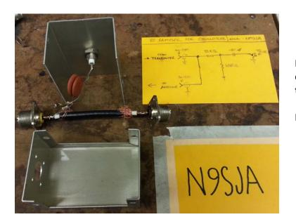
My build of Bob's RF sampler circuit. I did not have the correct capacitor so I used 2 .01 mfd caps in parallel for the .02 value.
